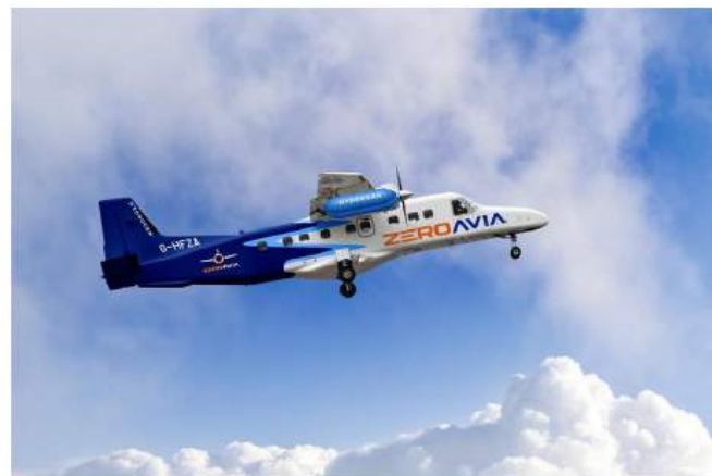
ZeroAvia is modifying the 19-seat Dornier 228 into a hydrogen fuel-cell propulsion testbed.
